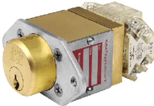
The Type TPS interlock is a key actuated switch utilizing two tandem mounted Square D Class 9001 KA1 contact blocks and is designed for back panel mounting (sub panel). The TPS can be installed so the lock cylinder will protrude 5/8" or flush mounted (by use of spacers).
